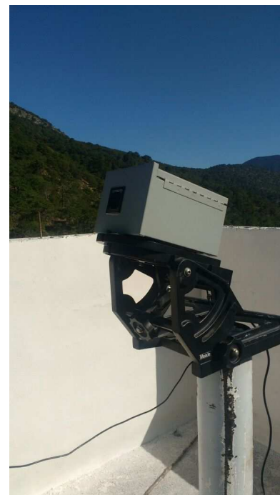
Figure 7. DIMM camera device for seeing measurements, currently installed at the UANL Solar Observatory.
