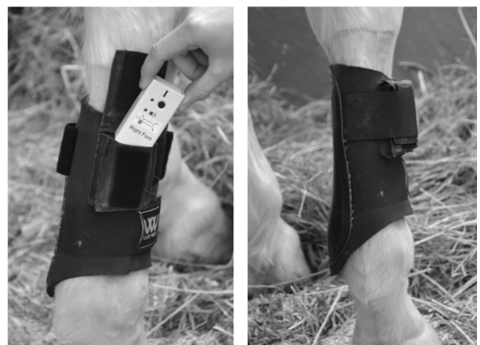
FIG 7: An exemplar of the custom fitted pouches, which are attached to the lateral aspect of each boot and strap to hold the IMU sensors firmly to reduce motion and to facilitate synchronicity with limb movement throughout the data collection period. Left: sensor is inserted into its pouch. Right: pouch is closed and Velcro strap is fastened over the sensor-pouch.
