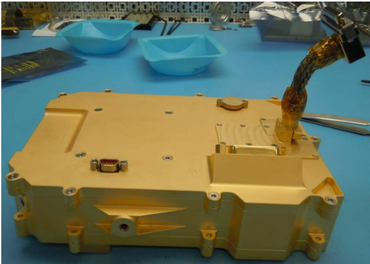
Figure 9 The Proximity Electronics housing containing the PE board for driving the FPA. The board is similar to that used on SIMBIO-SYS but with small modifications to the connector positioning so that the box could be mounted inside the rotation bearing. The box is roughly 20 cm in length.
