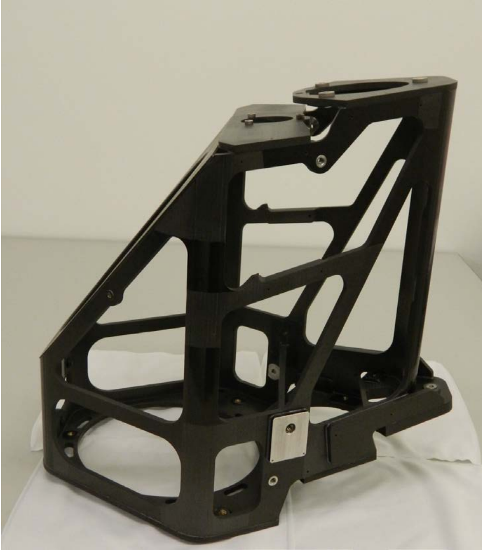
Figure 6 The CFRP structure of the telescope prior to mounting of the mirrors.
