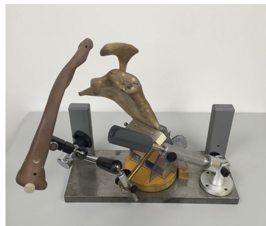
Fig. 1 Sawbone modelling. Specially designed holding device where a Sawbone Model was mounted. This model allows to simulate different ACJ dislocation as well as navigation in axial, sagittal and coronal direction according to measurement protocol
