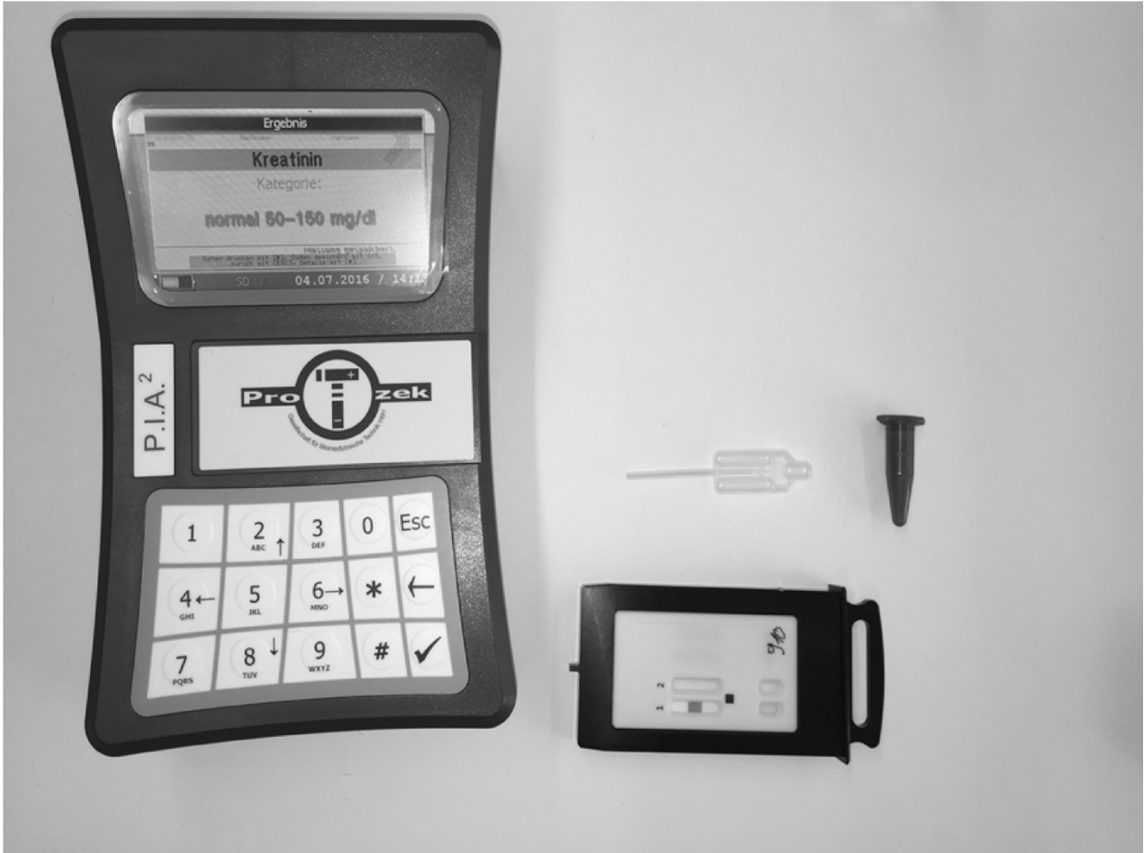
Figure 1 Automatic P.I.A.2 readout system from Protzek with a creatinine test cartridge, a microtube, and a 100 \mu L pipette for the dilution of the urine.
