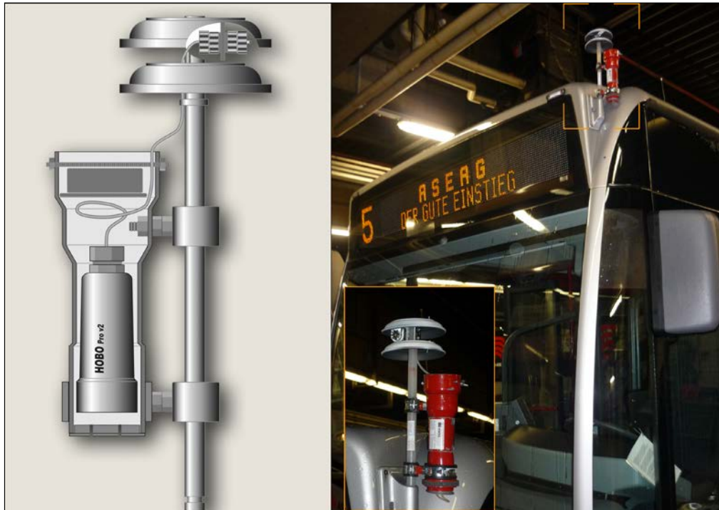
Fig. 1 Combined temperature and GPS logger mounted on a public bus (reprinted from Buttstädt et al. 2011)
