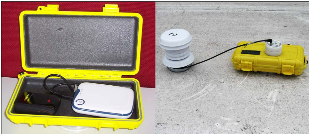
Fig. 6 Mobile measurement campaign in Hamburg. Left: Qstarz BT-Q1000XT GPS logger and Mobile Power Pack VT-PP-320b packed in the waterproof OtterBox 3000. Right: The instrumentation on the roof of a public transport bus. The logger is glued onto the OtterBox, the sensor is inside the radiation protection housing.
