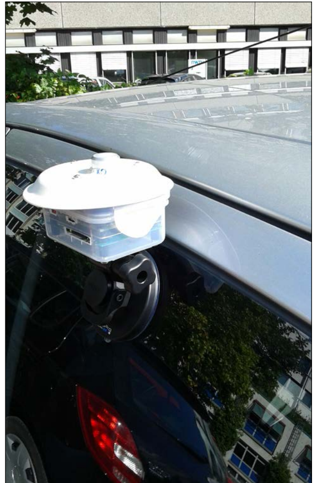
Fig. 5 Urbmobi 2.0 sensor installed on a car
