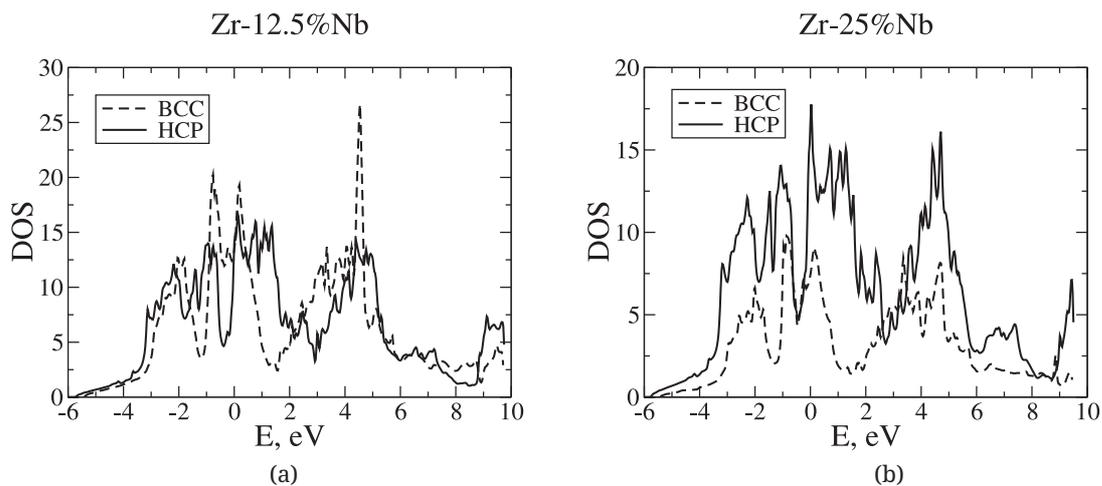
**Figure 4.** Dependencies for electronic densities of states (DOS) versus the energy measured from the Fermi energy for: (a) Zr-12.5%Nb alloy; (b) Zr-25%Nb alloy in the case of HCP lattice (solid curves) and BCC lattice (dashed curves).
