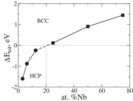
**Figure 3.** The difference in the total energy of HCP and BCC  $\Delta E_{\text{tot}}(\text{at.\%Nb})$  structures in eV for the unit cell of 32 atoms as a function of the niobium concentration in percentage for alloys Zr-Nb.
