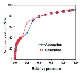
Fig. 8 CO<sub>2</sub> adsorption/desorption isotherms at 194.7 K for CFA-9.
