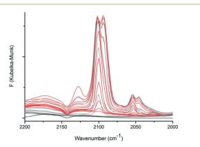
Fig. 11 In situ DRIFT spectra of CFA-9 recorded in 20 °C steps upon cooling from 100 °C to -100 °C under a CO atmosphere (red lines) and subsequent heating from -100 °C to 100 °C under an Ar atmosphere (gray lines). The DRIFT spectrum of KBr at -60 °C under a CO atmosphere (black line).
