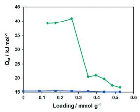
Fig. 10 Dependencies of the isosteric heats of  $O_2$  (blue) and CO (green) adsorption on the loading for CFA-9.
