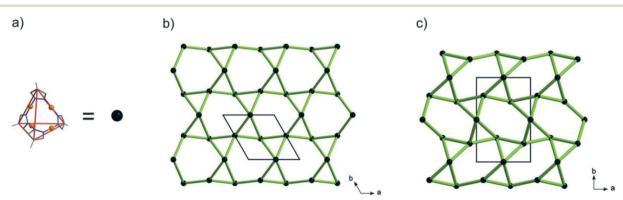
Fig. 4 (a) Simplified diagram of the SBUs of CFA-9. Topological representation of lp-CFA-9 (b) and np-CFA-9 (c).
