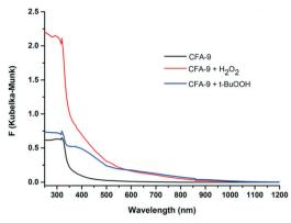
Fig. 12 UV-vis spectra of CFA-9 at room temperature. Black line – CFA-9, red – CFA-9 oxidized by  $H_2O_2$ , blue – CFA-9 oxidized by t-BuOOH.
