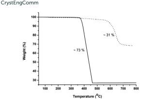
Fig. 6 Temperature-dependent weight loss of CFA-9 under flowing nitrogen (dashed line) and oxygen (solid line) gas.
