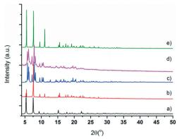
Fig. 5 Calculated and measured X-ray powder patterns for CFA-9. (a) Calculated pattern of lp-CFA-9; (b) measured pattern of lp-CFA-9; (c) calculated pattern of np-CFA-9; (d) measured pattern of np-CFA-9; and (e) dried sample re-solvated by DMF.
