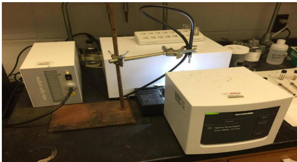
Figure 3. Agilent 8454 diode array UV-vis spectrophotometer (right) and SOLA light engine with the Light (left).
