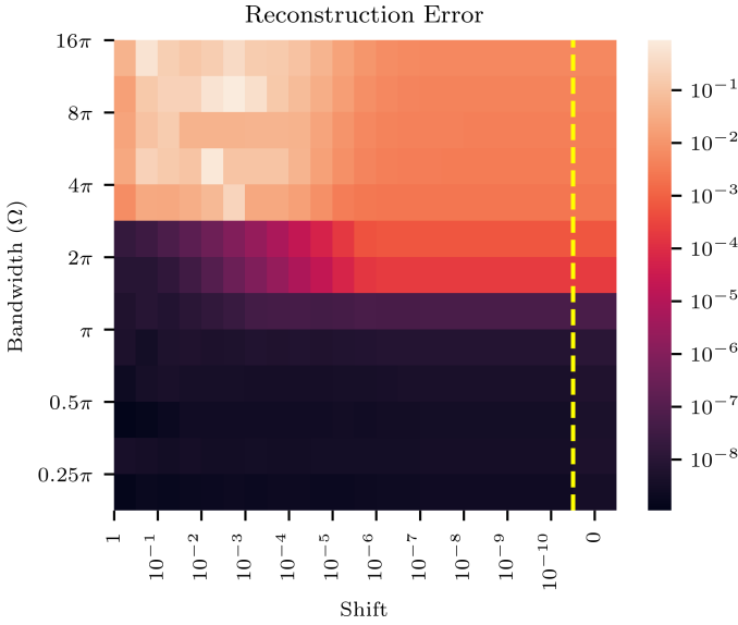
Fig. 10: Reconstruction error plotted as a function of bandwidth and integrator shift. A hundred 2\Omega -bandlimited signals, where \Omega varies between \pi/4 and 16\pi are generated and subsequently sampled and reconstructed using two-channel time encoding and decoding. The TEM used has fixed parameters \kappa , \delta and b but variable integrator shifts. The mean-squared error is averaged over the hundred randomly generated signals and plotted as a function of bandwidth and shift. Although we have shown that the value of the integrator shifts should have no effect on the reconstructible bandwidth (23), very small shifts perform less well than shifts that are within the same order of magnitude as the threshold \delta . The rightmost column, separated by the dashed yellow line, shows the reconstruction error when a shift of zero is used. In other words, this is the reconstruction error when using single-channel time encoding and decoding.
