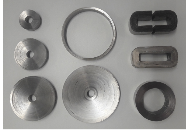
Fig. 9: Custom made core samples for experimental verification. First two columns: toroidal core samples that cover a wide A/R_m geometry range. Last column: cut and uncut U cores with identical size and their equivalent toroidal core
