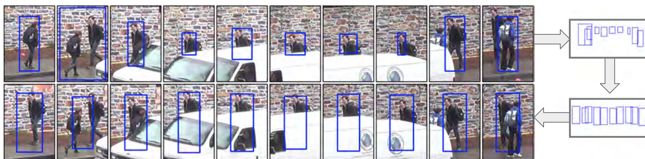
Figure 1. Keeping track in a difficult situation. Top row: Because of the occlusion created by the passing car, a tracker can easily return a trajectory that includes several identity switches. The corresponding bounding boxes inside camera’s field of view are shown on the right. Bottom row: Our algorithm not only eliminates identity switches but also regresses to a set of much tighter bounding boxes. In this example our algorithm did it solely on the basis of simple geometric features without requiring the use of appearance information.
