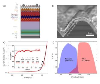
Figure 1. (a) Schematic view of the perovskite/p-type c-Si bottom cell. (b) Secondary electron scanning electron microcopy image of the cross-section of the front side of the perovskite/silicon tandem solar cell. (c) J-V properties and maximum power point tracking of the tandem (aperture area of 1.42 cm²), (d) corresponding EQE spectra.
