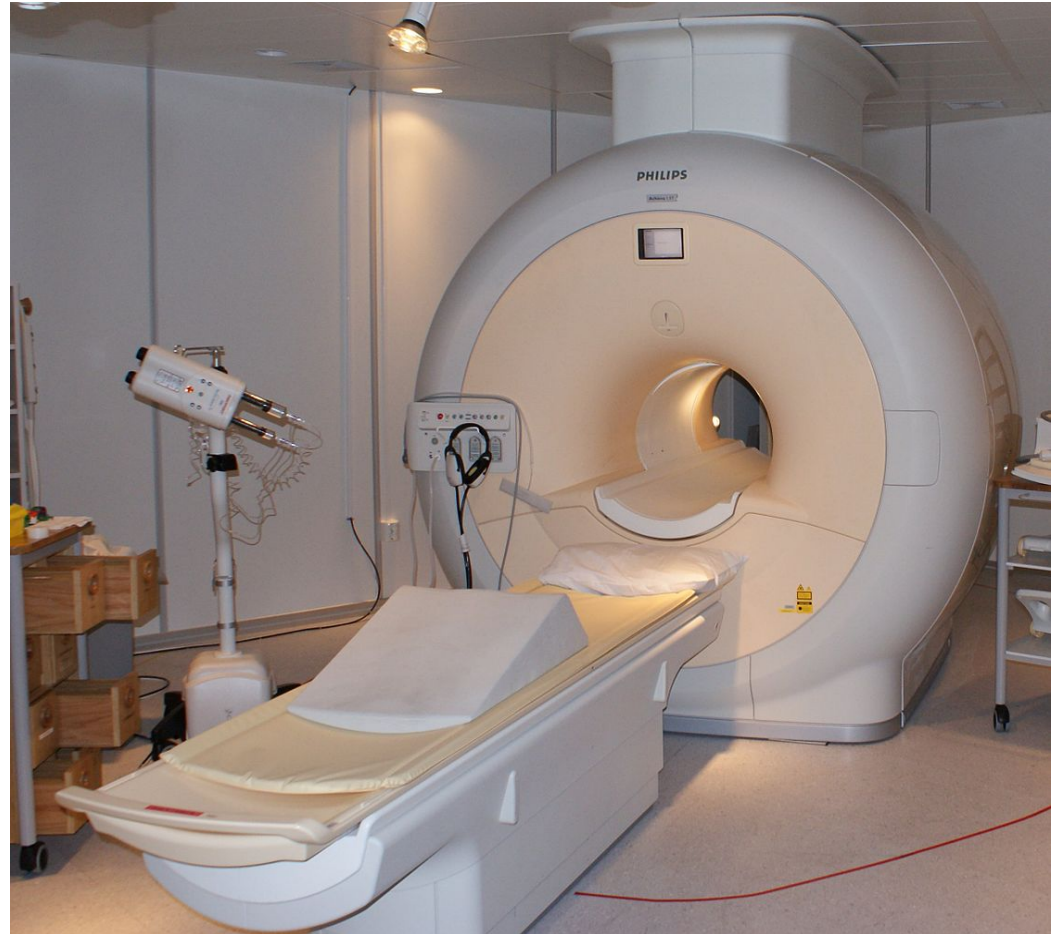
2b. Medicine: (Nuclear) Magnetic Resonance Imaging (typical 1.5 T, homogeneity \approx 0.2 ppm in \varnothing 36 cm)
