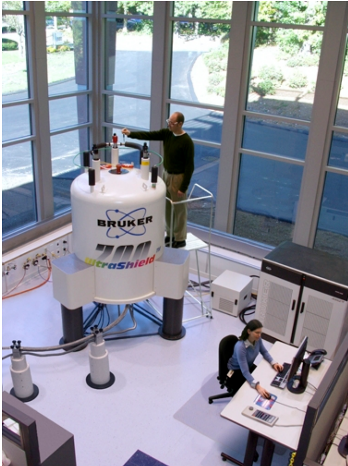
2a. Chemistry: NMR spectroscopy (up to 22 T / 900 MHz for H nuclei)
