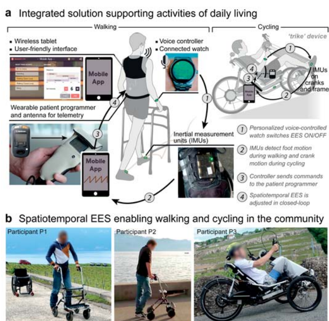
Figure 3.19 – Spatiotemporal EES in ecological settings. a , Tablet featuring a mobile App allows participants to select EES sequences, delivered in open loop or closed loop based on inertial measurement units (IMUs) located on both feet or attached onto the cranks and frame of a trike. b , Walking and cycling activities in ecological settings are enabled by spatiotemporal EES.
