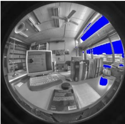
High Dynamic Range (HDR) vision sensor featured with fisheye lens generating false color images of an office room to identify potential glare sources (colored areas).
