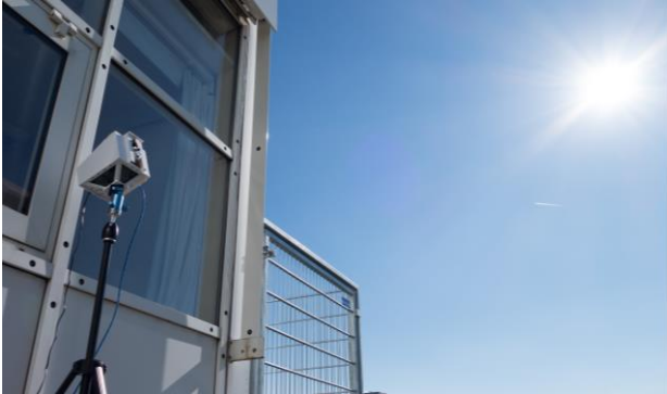
The embedded photometric device assessing work-plane illuminance based on sky monitoring.
