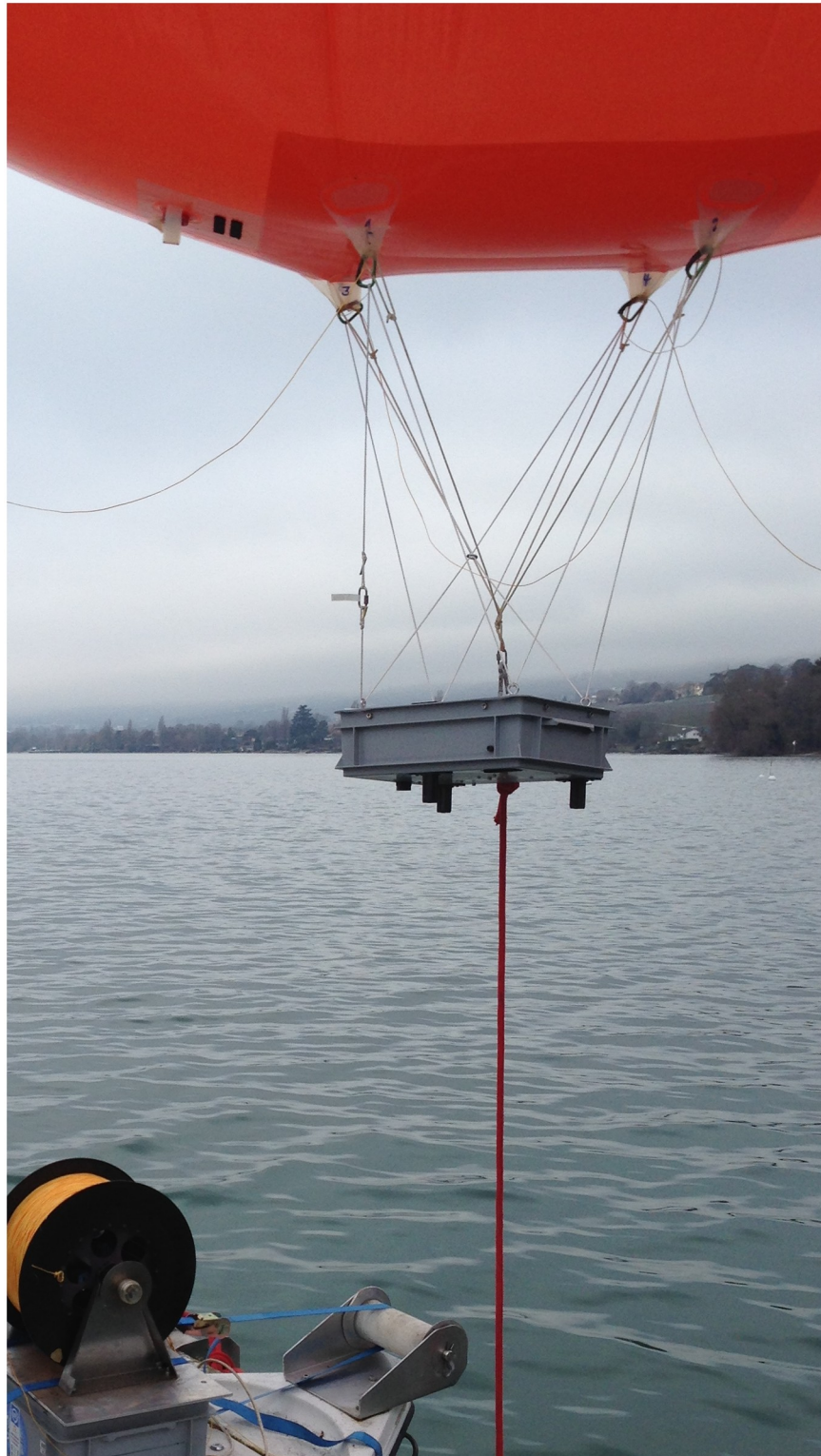
Fig 6. BLIMP system ready for deployment. The balloon is tethered to a winch, which controls its height. It carries the ImPROV instrument package installed in a grey box suspended by a Picavet harness.
