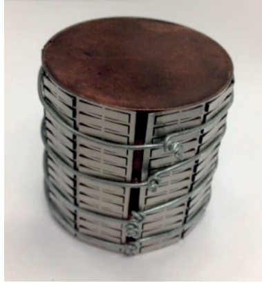
Figure 5.25 – Heat treatment of Cantilever beam foils.
