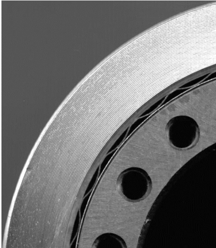
Figure 1.1 – A photograph of a partial sector in a journal foil bearing highlighting the sleeve, the bump foil, the top foil, and the rotor.
