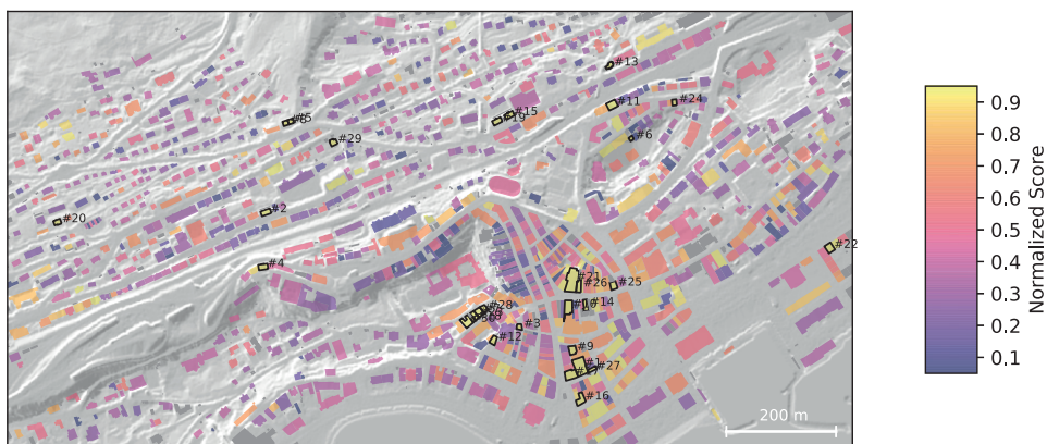
Figure 12.15 – Normalized score for the PV potential indicator (eq. (11.8)) using a minimum threshold of 650 kWh/kWp. The top-ranked buildings are highlighted with a black outline (# identifies the rank): they are located across the city, but a cluster can be seen in the central area. Results are more extensively described and discussed in Section 12.2.2.
