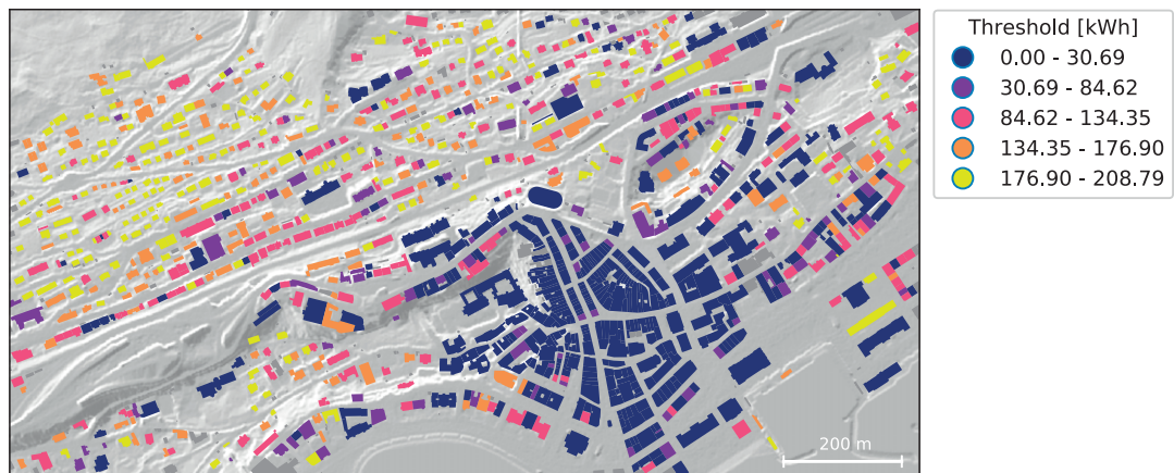
Figure 12.9 – Minimum electricity threshold per module for each building, as determined by the sizing heuristic (Algorithm 11.6). Buildings in the central areas have a low or null threshold, indicating that even considering all PV modules, Self-Consumption (SC) is greater than Self-Sufficiency (SS). The SC and SS values of these buildings are displayed in Figure 12.10b. Conversely, buildings in low-density areas present higher thresholds, meaning that some modules are discarded to reach a balance between the two indicators.
