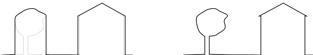
Figure 2.5 – Example of a 2.5D (left) and 3D (right) representation. Inspired by Peters [230]
