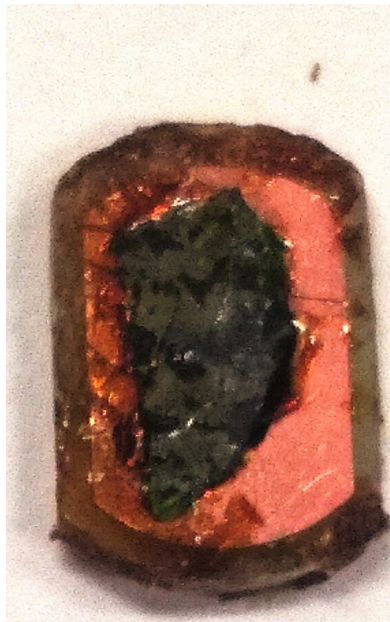
Figure 3.9 – Picture of Polished sample glued on the substrate with [111] direction perpendicular to the substrate plane
