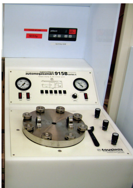
Figure 2.25 – The CPD machine at EPFL fabrication facility. For this project we use Automegasamdri®-915B critical point drier machine.
