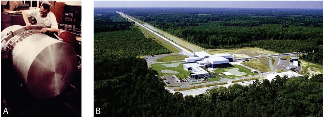
Figure 1.2 – Two generation of gravitational wave detectors. A) Joseph Weber with one of his aluminum cylinder resonant bar gravitational detector known also as Weber bars [Photo courtesy of AIP Emilio Segrè Visual Archives] B) Long interferometric gravitation wave detector such as LIGO [Photo courtesy of Caltech/MIT/LIGO Lab]
