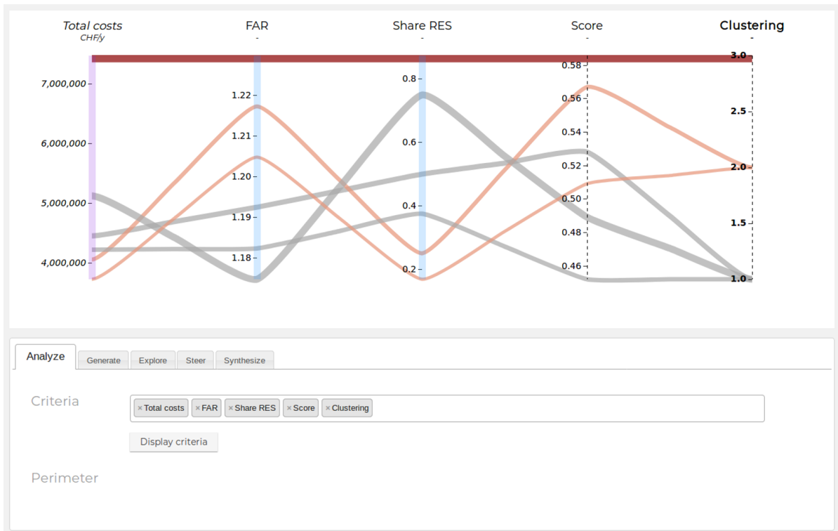
Figure 3.5 – Snapshot of the graphical user interface demonstrating several features of the SAGESSE methodology, including axis and polyline styling, multiattribute and cluster analysis results, and the axis selection menu. Line color indicates the belonging of a line to one of the three clusters (bold axis label), while line size is proportional to total costs (italic axis label).
