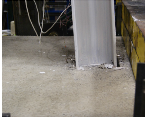
Figure 9 Minor spalling of slab near column after HS02-200%
