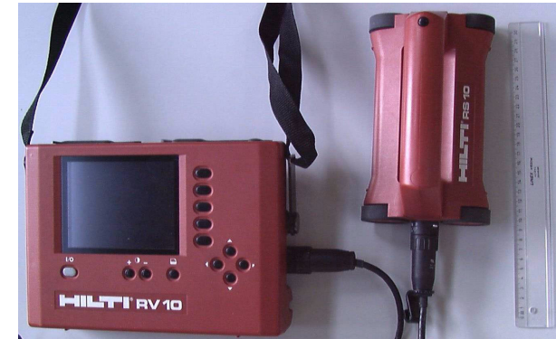
Figure 7.5: Ferrosan RV 10 monitor (left) and RS 10 scanner (right) (ruler length: 30 cm)
