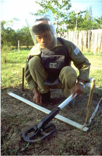
Figure 1.1: HALO Trust deminer in Cambodia, checking the ground with an Ebinger 420SI metal detector
