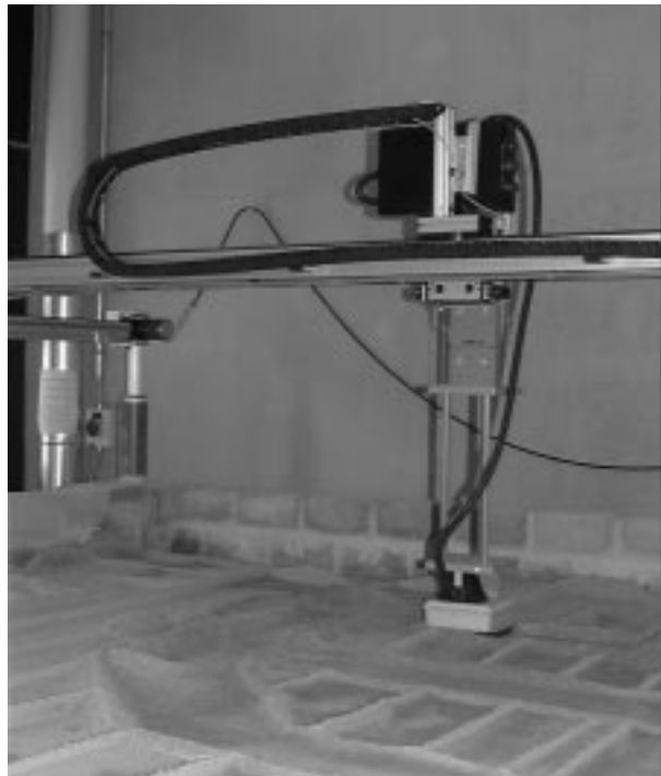
Figure 2: DeTeC test system: sand box, cartesian robot, 1 GHz antenna and radar head (top).
