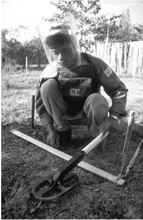
Fig. 1: HALO Trust deminer in Cambodia, checking the ground with an Ebinger 420SI metal detector
