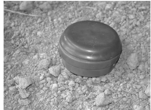
Fig. 3: Chinese Type 72 mine minimum-metal AP mine (78 mm large, 38 mm high)
