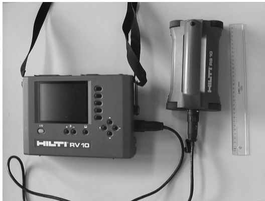
Fig. 4: Ferroskan RV 10 monitor (left) and RS 10 scanner (right) (ruler length: 30 cm) Fig. 5: Example of Metal Detector response at 5 increasing depths (general trend, differential sensor, line scan over the object)
