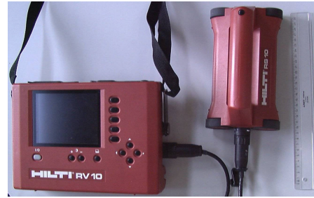
Fig. 8: Ferroskan RV 10 monitor (left) and RS 10 scanner (right) (ruler length: 30 cm)
