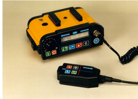
Fig. 4: An example of an advanced cover meter: Protovale CM9 CoverMaster®
