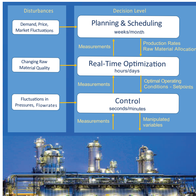
Figure 1.1 – Real-time optimization as a part of a multilayer control structure
