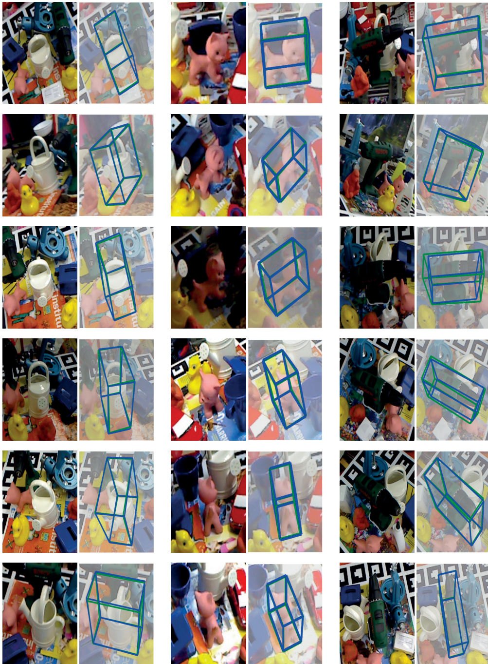
Figure 6.12: Example results of single shot pose estimation method on the LINEMOD dataset (II). (left) CAN, (middle) CAT, (right) DRILLER. The projected 3D bounding boxes are rendered over the image and they have been cropped and resized for ease of visualization. The blue cuboid is rendered using our pose estimate whereas the green cuboid is rendered using the ground truth object pose. Note that the input image dimension is 640 \times 480 pixels and the objects are often quite small. Noticeable scene clutter and occlusion makes these examples challenging.
