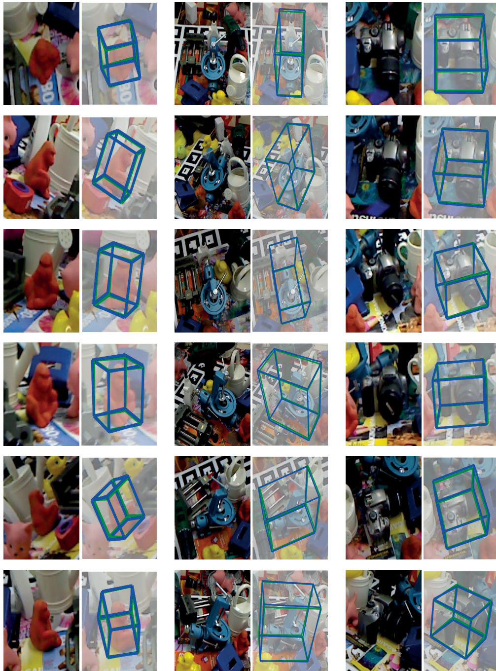
Figure 6.11: Example results of single shot pose estimation method on the LINEMOD dataset (I). (left) APE, (middle) BENCHVISE, (right) CAM. The projected 3D bounding boxes are rendered over the image and they have been cropped and resized for ease of visualization. The blue cuboid is rendered using our pose estimate whereas the green cuboid is rendered using the ground truth object pose. Note that the input image dimension is 640 \times 480 pixels and the objects are often quite small. Noticeable scene clutter and occlusion makes these examples challenging.
