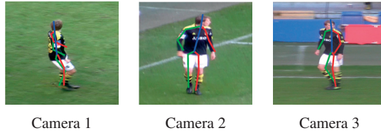
Figure 3.8: Results of our RSTV-Regression approach on KTH Multiview Football II. The 3D skeletons are recovered from Camera 1 images and projected on those of Camera 2 and 3, which were not used to compute the poses.
