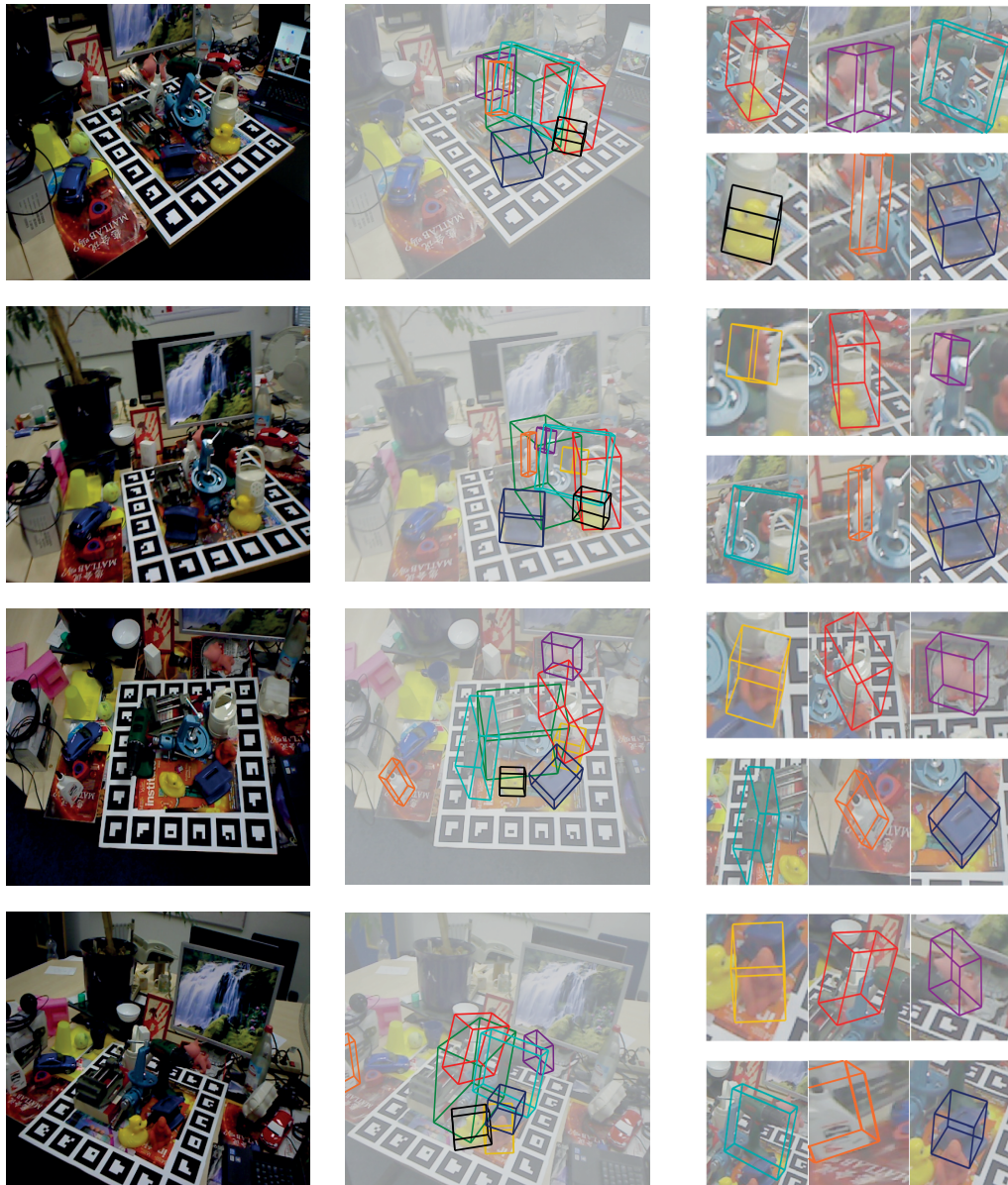
Figure 6.9: Results of our single shot pose estimation method on the OCCLUSION dataset (I). Our method is quite robust against severe occlusions in the presence of scene clutter and rotational pose ambiguity for symmetric objects. (left) Input images, (middle) 6D pose predictions of multiple objects, (right) A magnified view of the individual 6D pose estimates of six different objects is shown for clarity. In each case, the 3D bounding box is rendered on the input image. The following color coding is used – APE (gold), BENCHVISE (green), CAN (red), CAT (purple), DRILLER (cyan), DUCK (black), GLUE (orange), HOLEPUNCHER (blue). In addition to the objects from the OCCLUSION dataset, we also visualize the pose predictions of the Benchvise object from the LINEMOD dataset. As in [152], we do not evaluate on the Eggbox object, as more than 70% of close poses are not seen in the training sequence. This image is best viewed on a computer screen.
