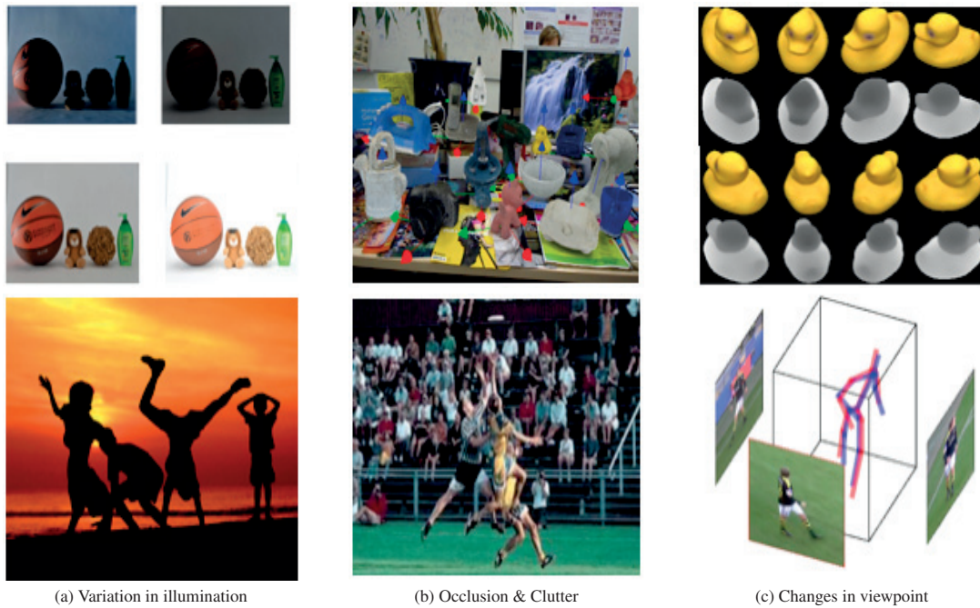
Figure 1.3: Challenges of 3D pose estimation for objects (top) and humans (bottom). 3D pose estimation is a challenging problem to solve. The challenges include variation in illumination, occlusion and clutter, variation of viewpoint and more generally the loss of depth information resulting from projection from 3D to 2D. Top row: (a) an image showing objects captured at different illumination conditions from the Phos dataset [212], (b) an image showing objects on a cluttered office desk from the LINEMOD dataset [69], (c) a 3D object viewed from different angles (adapted from the slides of [73]). Bottom row: (a) a group of people under low illumination conditions (retrieved from Flickr, photo credit: Nattu Adnan) (b) an image showing occluded ultimate frisbee players on a cluttered background (photo credit: Jon Hope), (c) a football player captured from different viewpoints and its 3D pose estimation result by [197].
