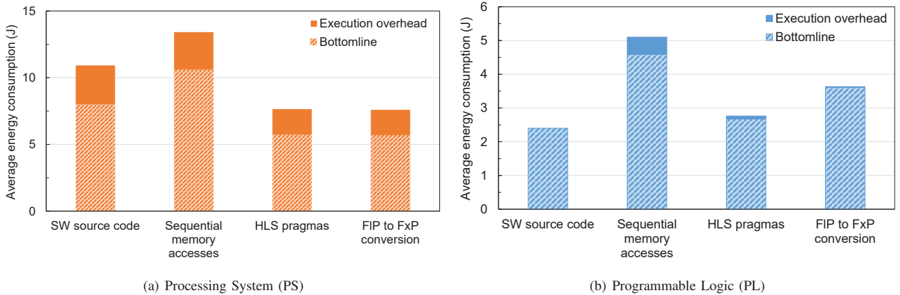
Fig. 8: Energy bottomline and execution overhead for PS (a) and PL (b).
