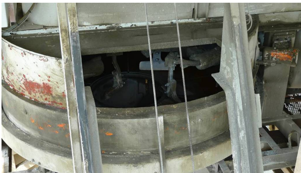
Figure 6: Concrete mixer used for the preparation of the UHPFRC.
