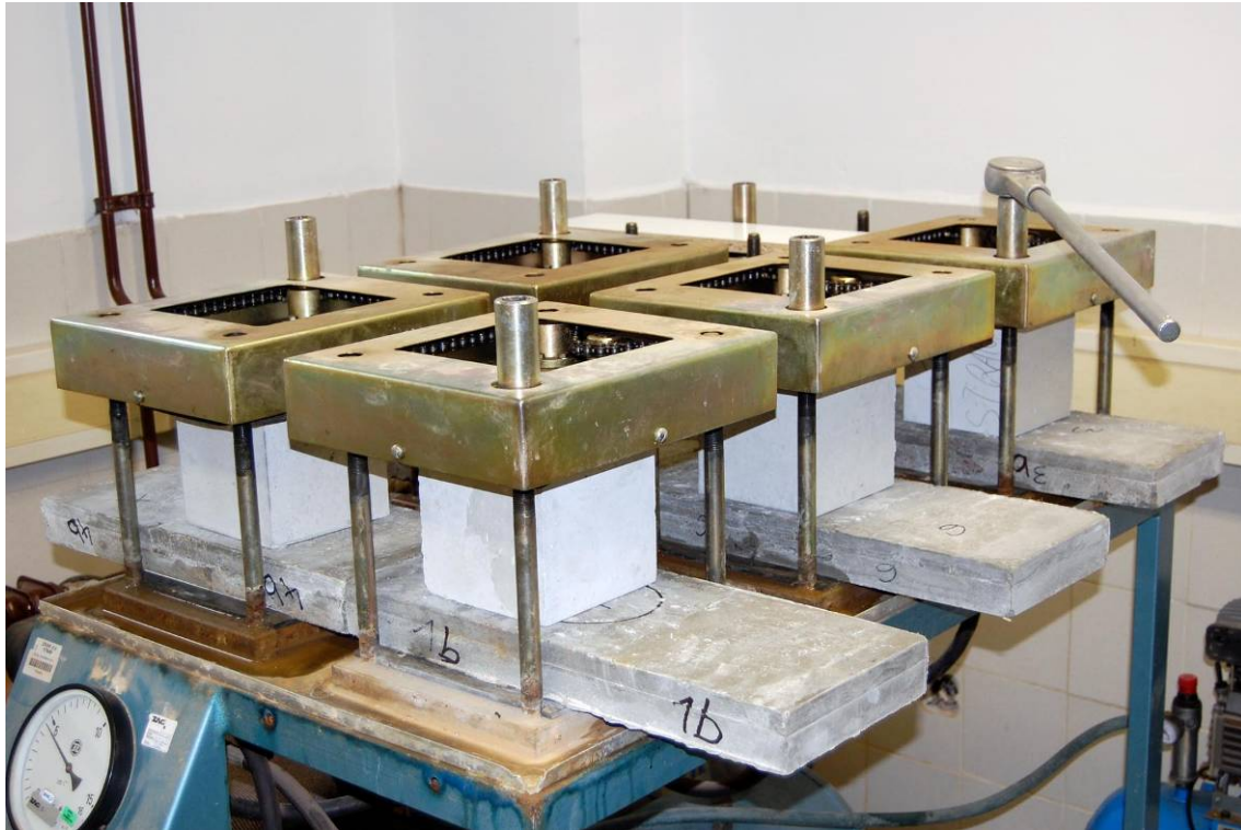
Figure 29: Depth of penetration of water under pressure test.
