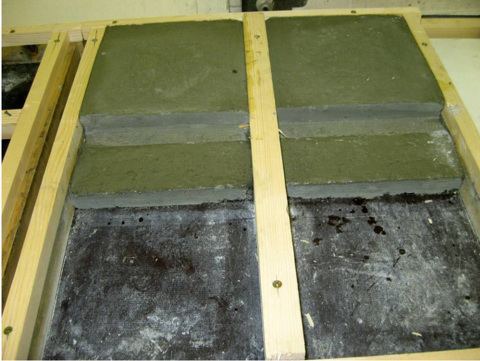
Figure 26: Joint before the second half casting.
