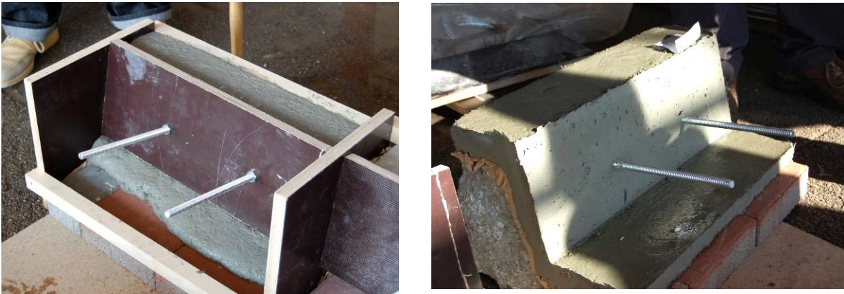
Figure 9: Trial tests for casting the inner faces of kerbs with an open formwork. Thick-
