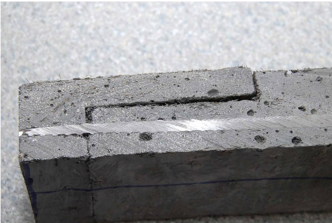
Figure 34: Failure mode of the concrete-reinforcement bond.
