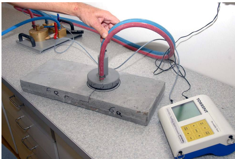
Figure 28: Air permeability test of the joints.
