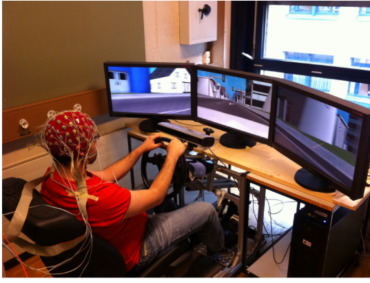
Fig. 2. Driving simulator used in the experiments. The subject drives a simulated vehicle through a simulated environment shown in three 3D screens while wearing a 64-channel EEG acquisition system.
