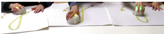
Figure 5: Driving the robot activity with 3 children. Each child drives their own robot with real-time haptic feedback when the robot is out of the letter's path.
