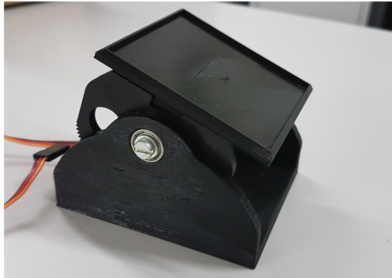
Figure 9: One-way tilt with interchangeable top plates.
