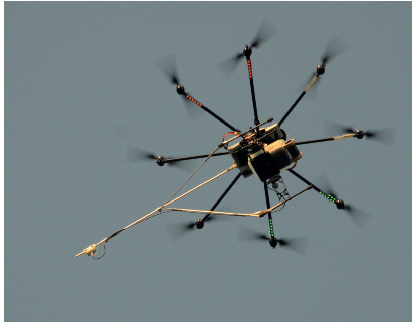
Figure 2.1 – Image of the UAV platform in stationary flight photographed from the ground. The fast-response pressure probe and the thermocouple are mounted at the extremity of a carbon fiber beam and at a distance of 115 cm from the UAV center in order to avoid the rotor downwash. The rest of the equipment is mounted on a platform below the main UAV body.
