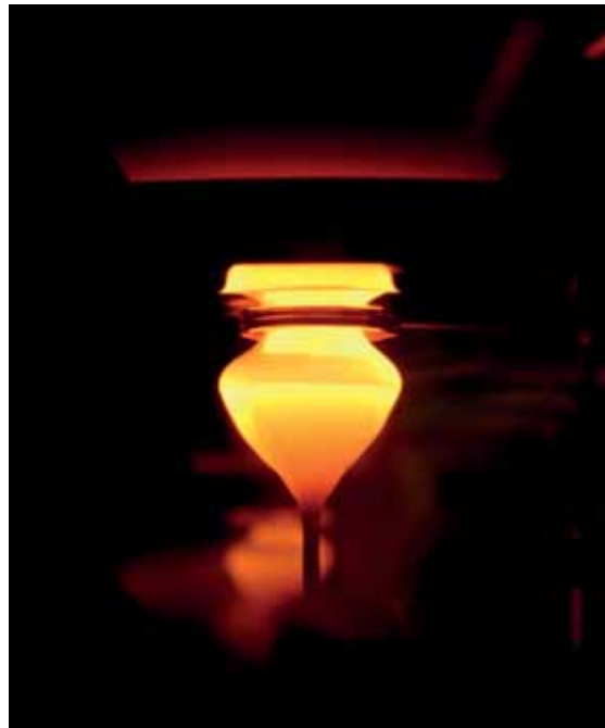
Figure 3.1 – Start of float zone crystal growth: Heating coil locally melts the polysilicon, attached to a thin top seed crystal layer [84]
