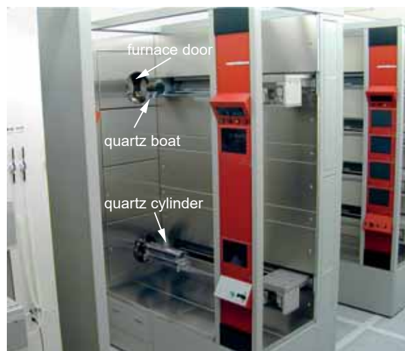
Figure 3.2 – Centrotherm LPCVD system: A loading arm containing wafers vertically placed on quartz boat, sits in front of LPCVD furnace door, with the reaction chamber recessed behind the wall
