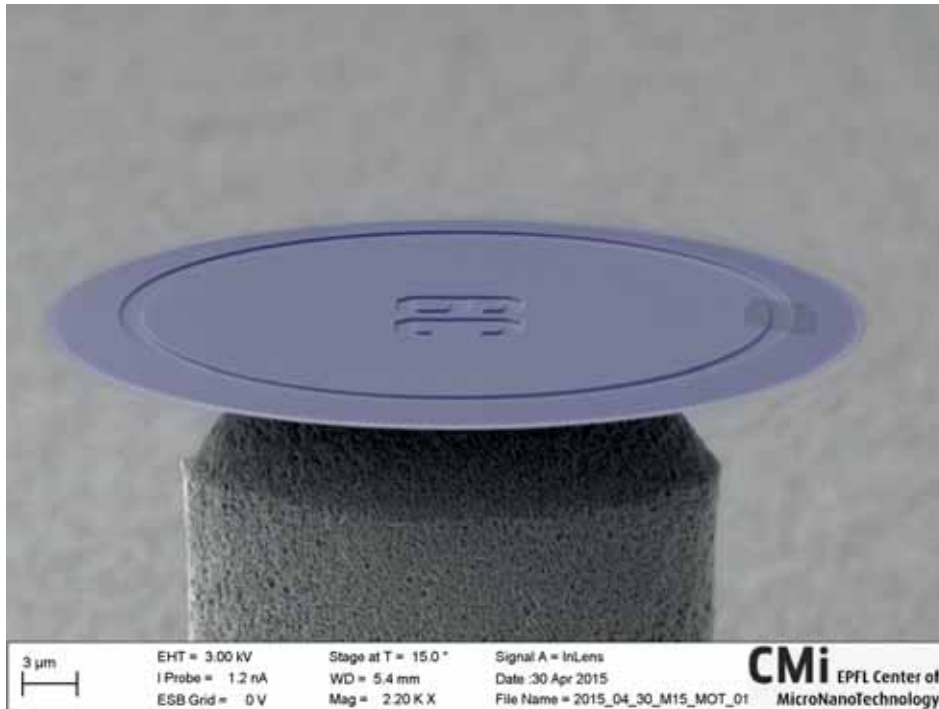
Figure C.5 – Possibility to use e-beam microdisks for 2D optomechanics: a version of the structure in fig. C.4 is modified to include a 50 nm deep and 1 μm wide channel around its perimeter (SiO 2 false colored to blue). The image is modified to show the concept of applying a flake of 2D material over this channel to create a suspended mechanical structure, where its motion would be optically coupled to the microdisk mode.
