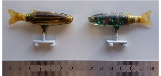
Fig. 3. Actuated biomimetic lure RiBot used in the experiments. Left: Lure with a zebrafish color pattern. The pattern was printed on the skin of the lure using decals. The pattern was then covered with latex to become waterproof. Right: Lure without any zebrafish color pattern. The PCB with all the electronic components that are used for the actuation of the caudal peduncle can be seen from the outside.
