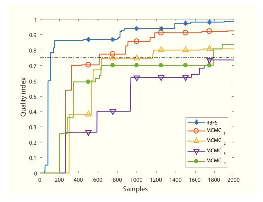
FIG. 16. Comparison of the candidate domain provided by 2000 samples generated using RBFS and four MCMC characterised by different proposal widths. MCMC<sub>1</sub> denotes the best parameter setting found after four attempts. Since RBFS does not require initial tuning, there is less risk of low-quality results.
