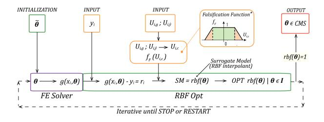
FIG. 6. Flow chart of the radial-basis function sampling (RBFS). (\*) For the Falsification Function refer to Figure 7.
