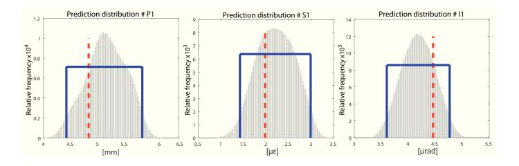
FIG. 18. Distribution of candidate-model-set predictions (PD) at three sensor locations (P1, S1 and I1) that have not been used for falsification. The uniform PDs for a 95% confidence and the CMS prediction distributions are plotted. For each sensor, the PD includes the measured value. The PDs have been identified using 2000 initial samples generated through RBFS.
