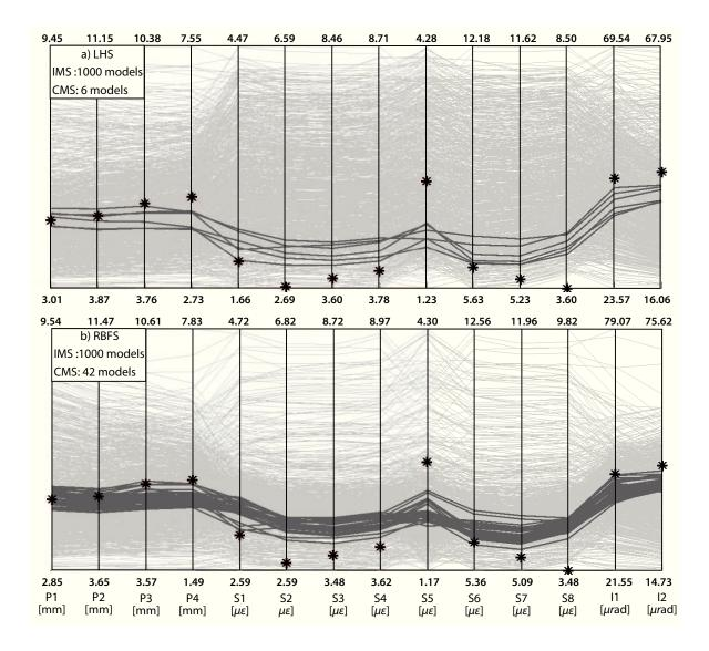
FIG. 11. Predictions of 1000 model instances generated using Latin hypercube sampling (LHS), top and radial basis function sampling (RBFS), bottom. Each vertical axis represents the prediction at the sensor locations defined in Figure 9. Predictions of the initial model set (IMS) (grey lines) and the candidate model set (CMS) (dark lines) are plotted. CMS-prediction thresholds are reported for each axis. Black asterisks (\*) represent the measured value at each location.
