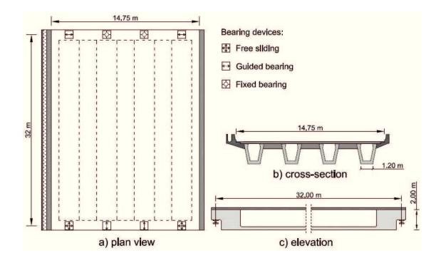
FIG. 8. Plan view a), cross-section b) and longitudinal profile c) of the bridge. The flyover is a 32-meter-long span reinforced-concrete bridge that consists of four precast beams with cast-in-place diaphragms at the abutments. The cast-in-place concrete deck connects all the beams and the two precast concrete barriers.
