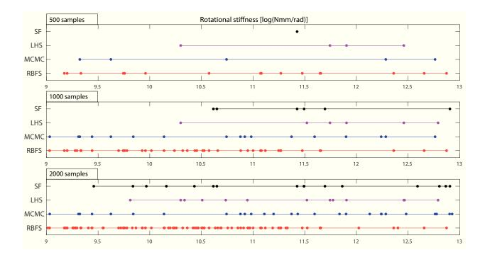
FIG. 13. Comparison of rotational stiffness values identified using RBFS, MCMC, LHS and SF. Falsification has been conducted considering three initial model sets that consist of 500, 1000 and 2000 samples. RBFS provides the largest CMS and the most effective exploration of the candidate domain, even with 500 samples.
