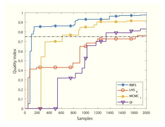
FIG. 17. Comparison of the candidate domain provided by 2000 samples generated using RBFS,  $LHS_0$ ,  $MCMC_1$  and SF. The main drawback of non-adaptive sampling is the slow exploration of the domain with increasing number of samples.
