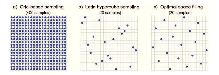
FIG. 1. Examples of sampling in a 2D domain using: a) grid-based sampling, b) Latin hypercube sampling (LHS) and c) optimal space-filling sampling (SF).
