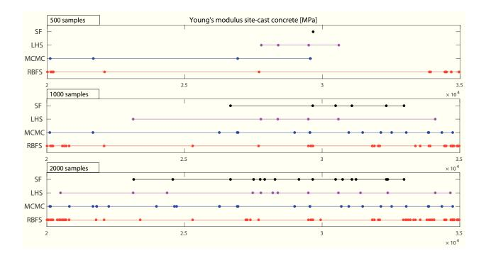
FIG. 14. Comparison of Young's modulus values for cast-in-place concrete, identified using RBFS, MCMC, LHS and SF. Falsification has been conducted considering three initial model sets that consist of 500, 1000 and 2000 samples. RBFS covers the entire candidate domain within 500 samples, performing better than MCMC.
