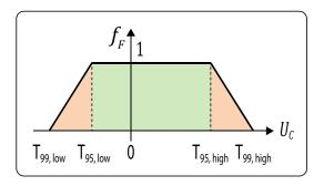
FIG. 7. The falsification function is defined by the combined uncertainties. Two triangular distributions are attached to the rectangular distribution to guide the search for optimal values.
