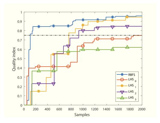
FIG. 15. Comparison of the candidate domain provided by 2000 samples generated using RBFS and four LHS.  $LHS_0$  denotes the default LHS-setting implemented in ANSYS. Three more populations ( $LHS_1$ ,  $LHS_2$  and  $LHS_3$ ) have been generated through a random selection of the sampling seed. The quality of candidate domain exploration provided by LHS is affected by the random choice of the seed value.
