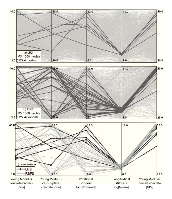
FIG. 12. Parameter values describing 1000 model instances generated using LHS and RBFS. Each vertical axis represents a parameter. Initial model instances (grey lines) and candidate models (dark lines) are plotted and initial values of each parameter are given for each axis. The comparison of candidate models is shown in c).
