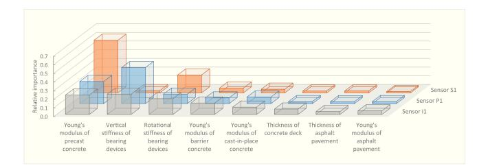
FIG. 10. Relative importance of parameters  $\theta$  on model predictions at three sensor locations (P1, S1 and I1).
