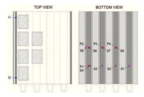
FIG. 9. Top and bottom views of the flyover. The truck configuration is shown along with the position of two inclinometers (I), four deflection prisms (P) and eight strain gauges (S).
