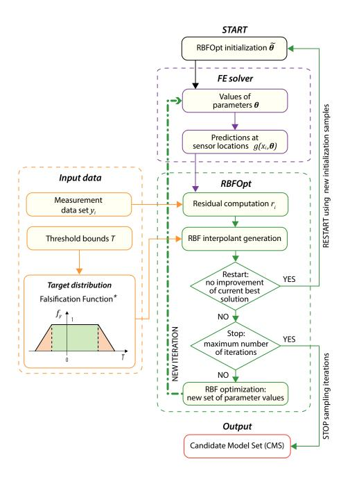
FIG. 5. General framework of the radial-basis function sampling (RBFS). (\*) For the Falsification Function refer to Figure 7.
