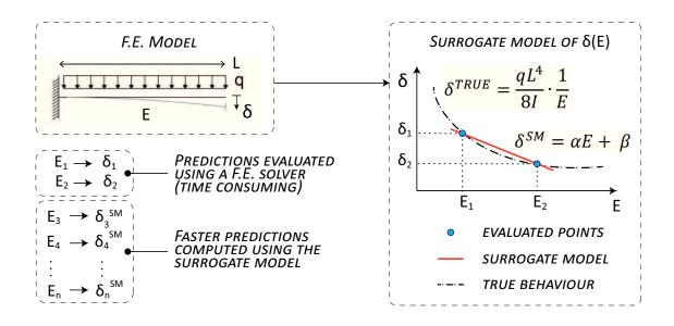
FIG. 3. Surrogate-model of the structural behaviour. A Surrogate models (SM) is used to speed up the computation of the maximum deflection  $\delta$  in a cantilever beam. To build the SM, first two predictions are provided by the FE solver (blue points). Then, additional predictions are calculated using the SM since it computes faster than the FE solver.
