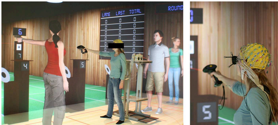
FIGURE 1 | Experimental Setup. (Left) Subjects were standing in the immersive projection system and were able to interact with the system using an ART Flystick. (Right) Subjects were wearing a high-density 64 channels EEG cap.
