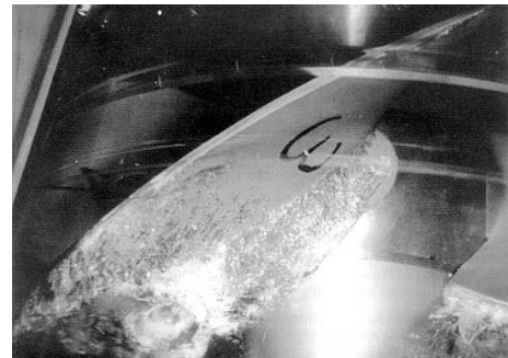
Fig. 30 Hub cavitation development for a Kaplan runner
