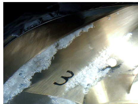
Fig. 31 Tip clearance and hub cavitation for a Kaplan runner
