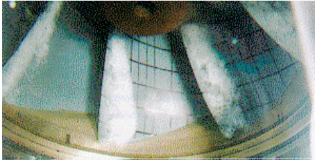
Fig. 10 Leading edge cavity development in a storage pump impeller, Q < Q_0 , during model testing.
