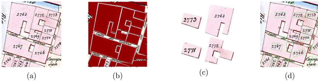
Figure 2: Sample of results : (a) original image, (b) polygon approximation of parcels, (c) extracted parcels and (d) identifiers localization
