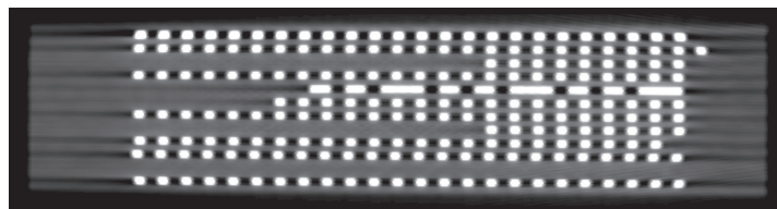
Fig. B.10 Planar transformer PCB windings cut view is in the zy plane, in the middle of the bottom horizontal section of Fig. B.9, obtained by a micro Computed Tomography (CT) scanner [165]. Only 11 copper layers are visible here, since the connection layer ((k) in Fig. B.9) has no track in the region of the cut.
