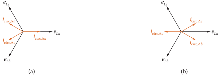
Fig. 4.12 Reactive currents creation to achieve cancellation on the bus: (a) positive case and (b) negative case of a required action for the vertical balancing in phase-leg a . The quadrature in phase-legs b and c is clearly visible.
