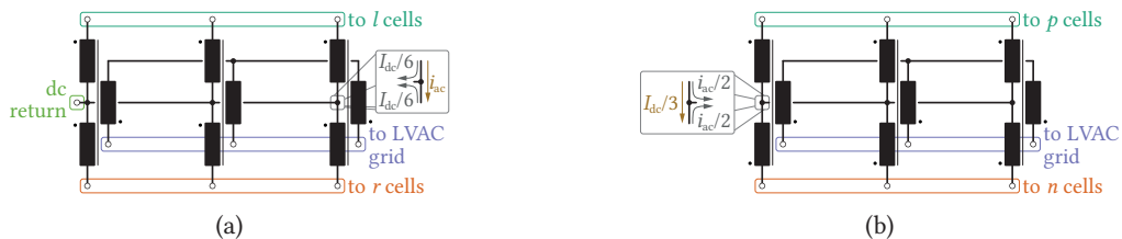
Fig. 6.10 Multi-winding transformer configurations to achieve the dc bias cancellation in the magnetic material, along with the current composition: (a) for the case of parallel-connected branches and (b) for the case of series-connected branches. The l and r cells are defined as the set of cells from the left and right parallel branch, as shown in Fig. 6.11(a).
