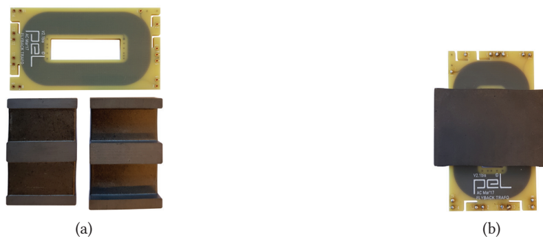
Fig. 9.7 Realized planar transformer: (a) separate elements before assembly and (b) assembled transformer. The PCB is 61.6 mm × 34.1 mm × 3 mm and the ferrite core 43.2 mm × 27.8 mm × 13.6 mm. The total planar transformer footprint is 61.6 mm × 43.2 mm. The pin numbers on the planar transformer PCB are matching the ones in Fig. 9.6 .
