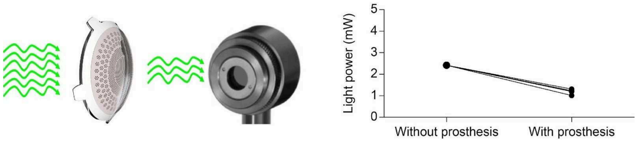
Supplementary Figure 6 | Optical absorption. Light absorbance/transmittance of POLYRETINA has been evaluated by using a green LED (565 nm, 2.42 mW). Light has been measured with a power meter (PD300-R Juno, Ophir Optronics Solutions Ltd.). The retinal prostheses ( N = 4 ) have been inserted in the light path and the light power has been compared with respect of the condition without the prostheses.
