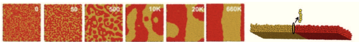
Figure 18. Simulation snapshots of phase separation in symmetric ( \varphi = 0.5 ) mixture at surface density of r = 4.0 of immiscible ( \Delta a = 15 ) surfactants. The surfactants have the same molecular length. The number in the top right corner is the time step at which the snapshot was taken, where K refers to thousands and M to millions of time steps[68].
