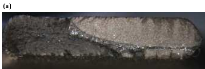
Figure 4: Fatigue fracture surface of the specimen loaded at 600 MPa (R=-1). (a) Global fracture surface showing the fatigue surface, (b) initiation zone identified at the surface of the specimen.
