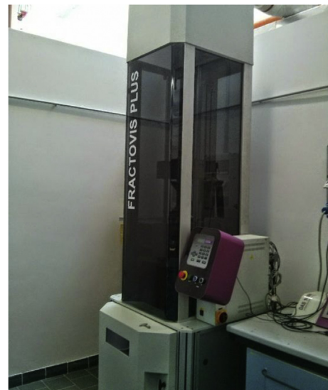
Fig. 6. Mechanical impact test stand.
