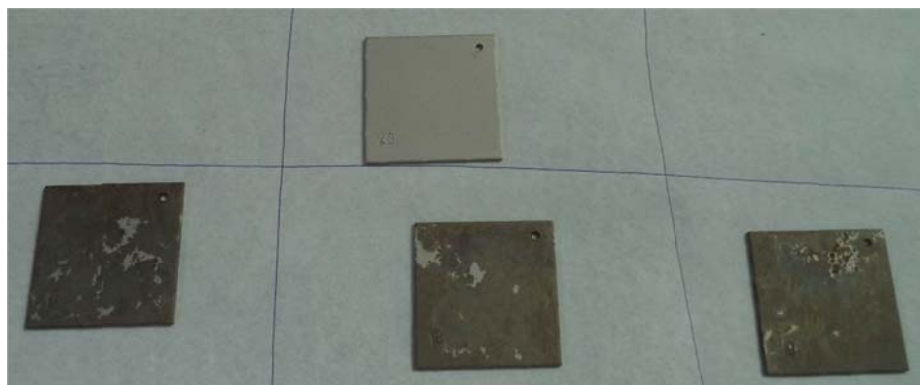
Figure 11. Aluminium specimens coated with Ni electroless coating. On the top, the reference, on the bottom, the three tested specimens.
