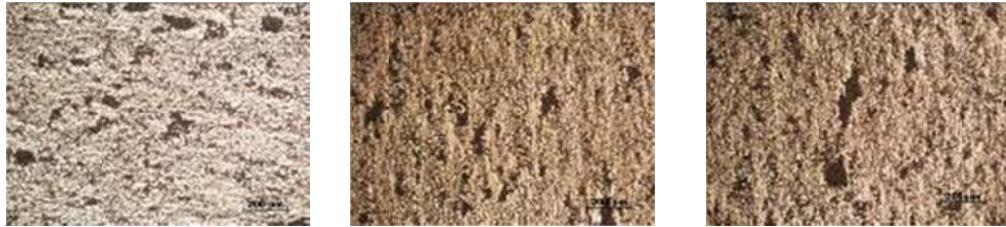
Specimens after corrosion test
