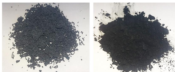
Figure 1. Expanded graphite – EG (left) and powder graphite – PG (right)
