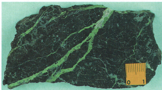
FIG. 4. Detail of the uvarovite veins in hand sample. Massive chromitite (black) is cut by millimetric veins of uvarovite (dark green). Calcite crystals (white) occur in the central part of these veins. The interstitial areas between chromite grains are filled by clinocllore (grey).
